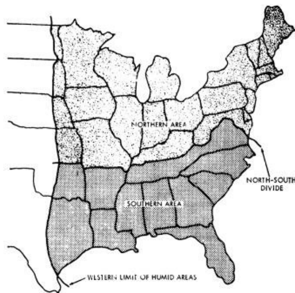
Figure 1 – Key map for drainage curves (Humid areas for eastern USA where surface drainage may be needed)
